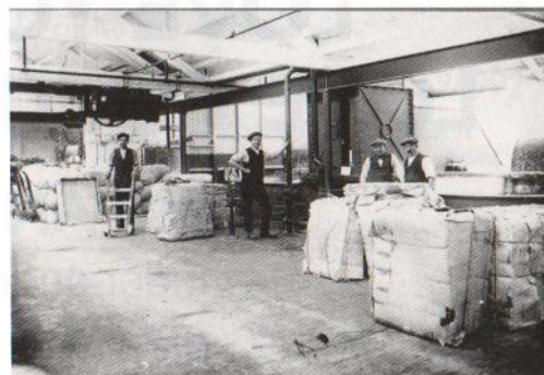
2. In 1935, when the majority of these images were made, paper was made from wood paper pulp bought in in packages – as seen here. The dried pulp was soaked in water tanks to form a thick paste which was progressively dried by passing it through heated rollers. The image shows the first stage in the papermaking process.
