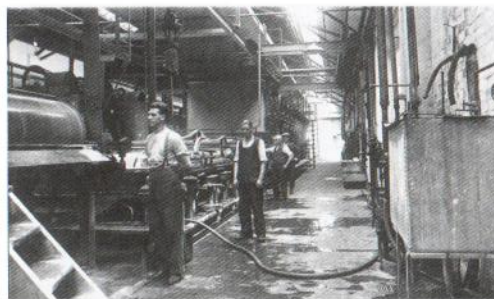
4. A papermaking machine – almost 100 feet long- was used to progressively dry and roll the wood pulp. The process began with the paste laid onto a mesh, rolled and then passed through the 100 feet of rollers to the point where it could be taken off as dried paper.
