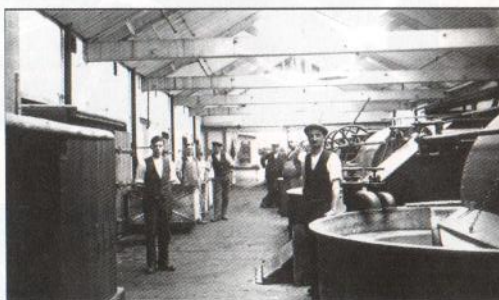
3. The dried pulp was pulverized in water tanks with powered beaters to create the paste which was then processed.
